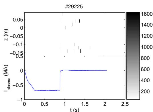
Figure 1: *Intensity of the signal in counts from channels at the laser wavelength together with the plasma current signal, showing no dust is present before the disruption.*
