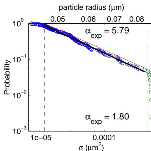
Figure 3: *Experimental cumulative distribution function of particle cross sections and radii using the Rayleigh approximation in the central spectrometer.*
