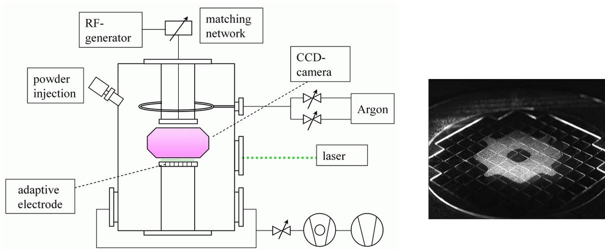
Figure 2: a) Experimental setup (PULVA-INP). b) Micro particles (Melamine formaldehyde,  $\varnothing$   $10\ \mu\text{m}$ ) levitated in an Argon-rf-plasma above the adaptive electrode. Negative bias voltage is applied to the central segment and to the segments surrounding the particles.
