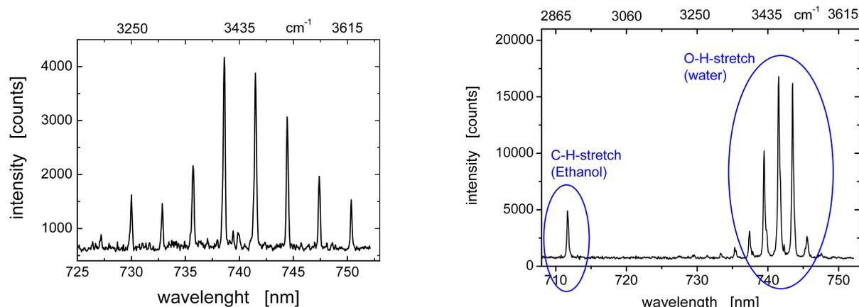
Figure 1: Cavity enhanced Raman spectrum from: a) a water droplet ( $r = 24.5\mu\text{m}$ ), b) a water/ethanol droplet ( $r = 35\mu\text{m}$ ).
