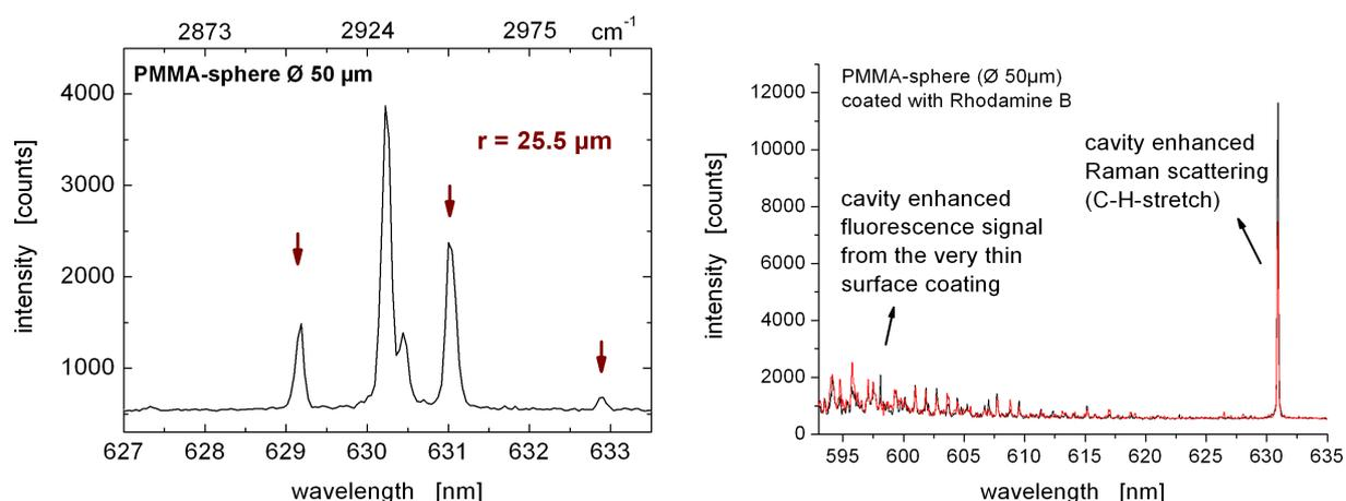
Figure 3: a) Cavity enhanced Raman spectrum from a PMMA-sphere. b) Spectrum from a polymer sphere ( $\varnothing 50 \mu\text{m}$ ) coated with Rhodamine B. The spectrum shows cavity enhanced Raman scattering in the C-H-stretching region at a shift of ca.  $2900 \text{ cm}^{-1}$  and also enhanced fluorescence from the dye covering the surface.
