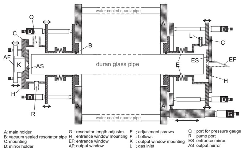
Figure 1: Sketch of the FIR resonator.
