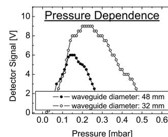
Figure 2: Influence of the laser medium gas pressure on the FIR signal ( $\lambda = 170.58 \mu\text{m}$ ) for two waveguide diameters.
