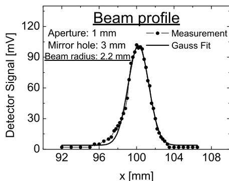
Figure 3: Beam profile of the  $\text{CH}_3\text{OH}$   $170.58 \mu\text{m}$  line at 55 mm distance. Beam radius: 2.2 mm.
