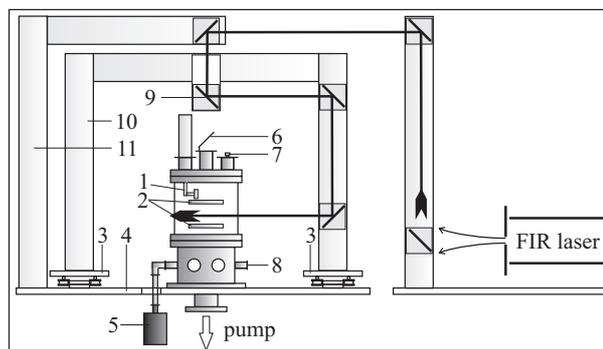
Figure 5: Sketch of the experimental setup. Labels: 1: dust dispenser, 2: electrodes, 3: guide rail, 4: table, 5: pressure gauge, 6: mirror, 7: rf connection, 8: different ports, 9: mirrors, 10: rotating mirror support, 11: fixed mirror support.
