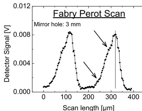
Figure 4: Fabry-Perot-Scan of the  $396.63 \mu\text{m}$  line of  $\text{HCOOH}$  shows three modes.
