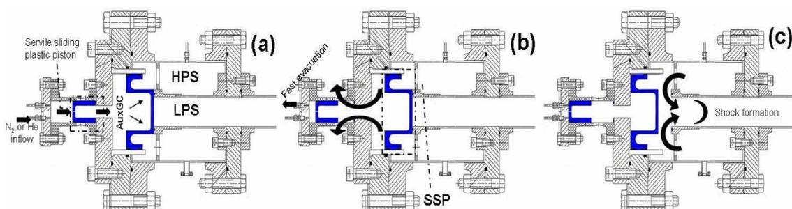
Fig. 2 – Principles of shock wave formation for the diaphragmless shock tube: (a) sealing mode via auxiliary gas inflow, (b) fast evacuation of auxiliary gas, and (c) shock wave formation.
