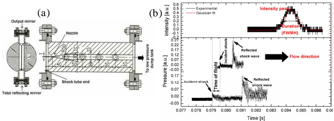
Fig. 3 – (a) supersonic nozzle section-infrared laser cavity assembly. (b) Sample of pressure histories (at the bottom) and  $10.6\text{-}\mu\text{m}$  laser radiation (at the top).
