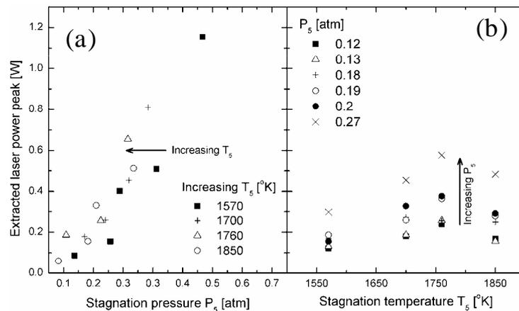
Fig. 4 – Peak power output of the  $10.6\text{-}\mu\text{m}$  laser radiation vs. (a) the stagnation pressure ( $P_s$ ) and (b) the stagnation temperature ( $T_s$ ).
