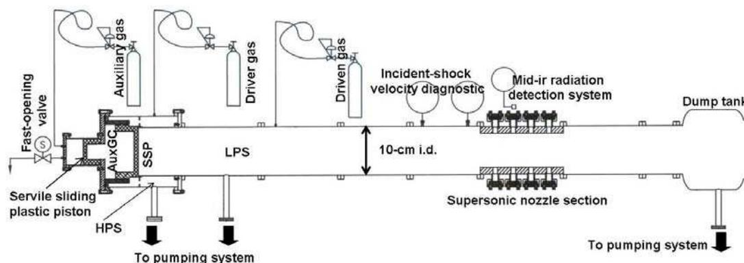
Fig. 1 – Overall drawing of the Kyushu University gas-dynamic laser, Kyudai GDL.
