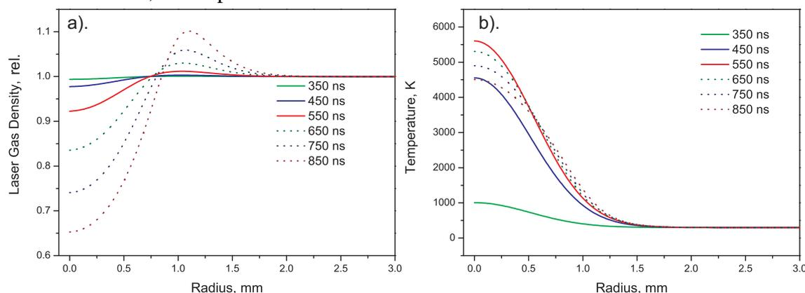
Figure 3: Laser gas density a). and temperature b). simulation (ion beam come at 300 ns).
