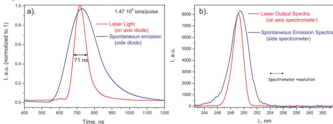
Figure 4: a). Time structure of the spontaneous emission and the laser pulse. b). Spectra of the spontaneous and laser emission, respectively, recorded with one the low resolution spectrometer.
