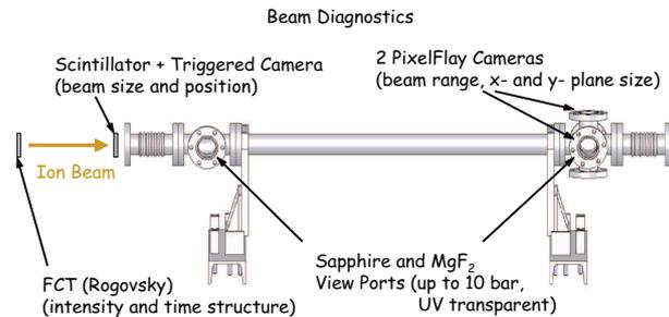
Figure 1: Laser stainless steel tube and heavy ion beam diagnostic.
