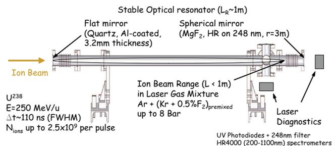
Figure 2: Stable optical resonator and laser light diagnostics.
