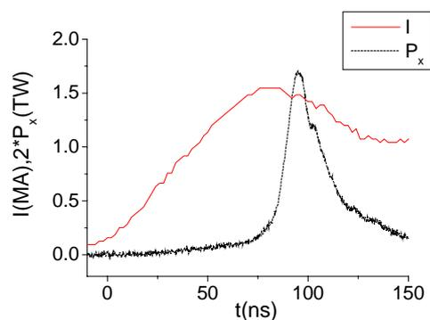
Fig.2 Typical X-ray power waveform obtained by XRPM together with current waveform in shot 03197. The load with a diameter of 8mm consists of 32 tungsten wires with wire diameter 5 $\mu\text{m}$ .
