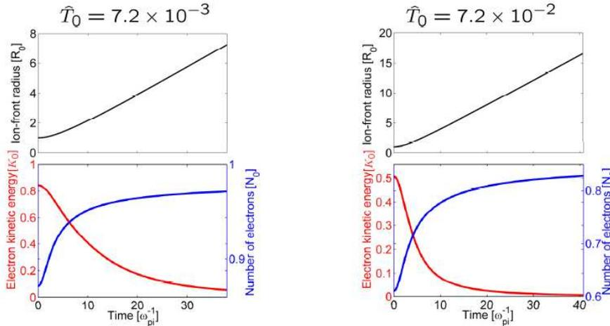
FIG. 3: Evolution of the number of electrons (blue) within the instantaneous radius of the ion front (black), and of the total kinetic energy of trapped electrons (red).
