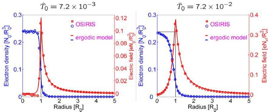
FIG. 1: Electron density (blue) and electric field (red), after the initial charging transient.
