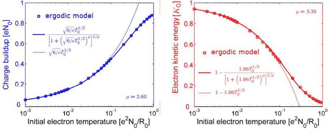
FIG. 2: Charge buildup within the ion core (blue) and total kinetic energy of trapped electrons (red) as functions of  $\hat{T}_0$ , after the initial charging transient. Circles refer to the present theory, while solid lines refer to the displayed fit laws. Thin lines show the power-law behaviours in the low-temperature regime.  $K_0$  is the initial total kinetic energy of the electrons.
