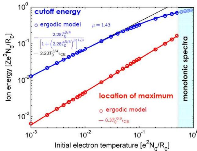
FIG. 5: Cutoff ion energy (blue) and location of the maximum in the ion energy spectrum (red) as functions of  $\hat{T}_0$ : circles refer to the present theory, while solid lines refer to the displayed fit laws.
