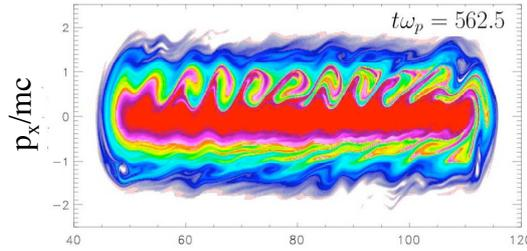
Fig. 2 : Electron phase space representation showing the SKSS development.
