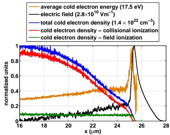
**Figure 1:** Demonstration of the ionization process in simulation. The 8  $\mu\text{m}$  long electron beam with the density  $10^{19} \text{ cm}^{-3}$  propagates (from the left) inside the plastic target, which begins at 8  $\mu\text{m}$ . Curves are normalized to the maximum values (see legend). The green and the red curves demonstrate the fraction of electrons produced by the field and the collisional ionizations respectively.
