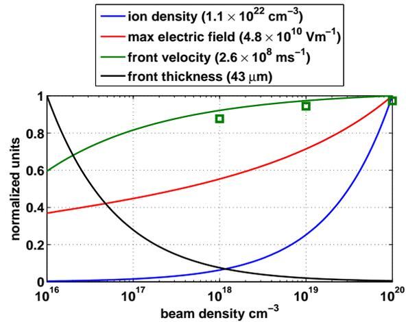
**Figure 2:** Dependence of the front velocity, maximum electric field, front thickness and ion density on the density of the electron beam calculated using the analytical model (markers represent the front velocity in simulation). Units normalized to maximum values (see legend).
