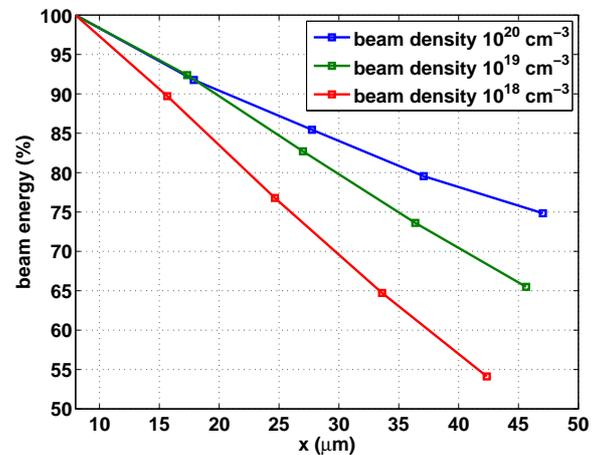
**Figure 3:** Energy losses of the beam in our simulations in % of initial energy versus the propagation distance. At 8  $\mu\text{m}$  beam enters the plastic target.
