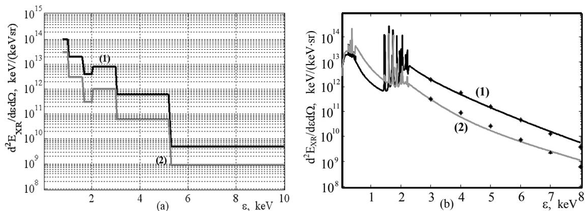
Fig.1. Experimental (a) and simulated (b) spectral distributions of X-ray radiation energy for massive aluminum (1) and multilayer (2) targets; symbol '\*' means exponential function with electron temperature  $T_e = 0.8$  keV.
