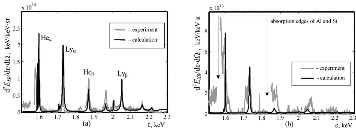
Fig. 2. X-ray radiation spectra in resonance lines of H-, He- like ions of aluminum for massive (a) and multilayer (b) targets.
