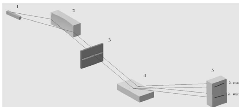
Figure 1. Layout of grazing incidence spectrograph. 1 – target, 2 – focusing mirror, 3 – spectral slot, 4 – diffraction grating, 5 – CCD-matrix.
