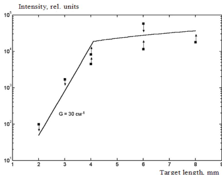
Fig 3. Dependence of XRL intensity on target length.
