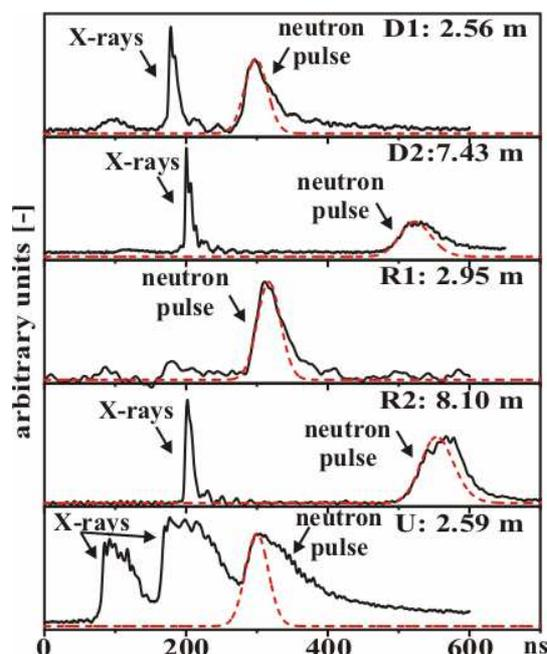
Fig. 3: The comparison of calculated (red) and measured neutron (black) signals detected behind the cathode (D), anode (U) and side-on (R).
