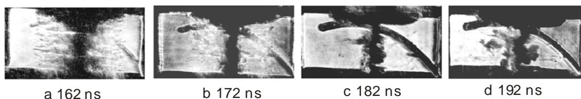
Fig. 2: Temporal evolution of the pinch phase imaged with laser diagnostic beam.
