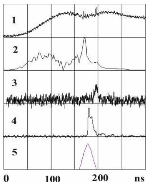
Fig. 1: Traces recorded in the shot No. 0506082: 1 – current, 2 – voltage, 3 – fast electrons above 50 keV detected axially behind the anode, 4 – hard X-rays above 100 keV, 5 – time of production of neutrons calculated using time-of-flight and MC methods.
