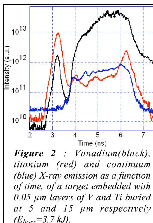
**Figure 2** shows a typical time evolution of the X-ray emission of the target recorded by the time resolved crystal spectrometer. This spectrometer was able to record the signals on every shot, including when the markers thickness was 0.05  $\mu\text{m}$ . The duration of the continuum emission is consistent with the laser duration. The two peaks around 3.2-ns are spurious direct X-rays.
