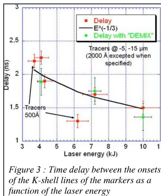
Figure 3 : Time delay between the onsets of the K-shell lines of the markers as a function of the laser energy
