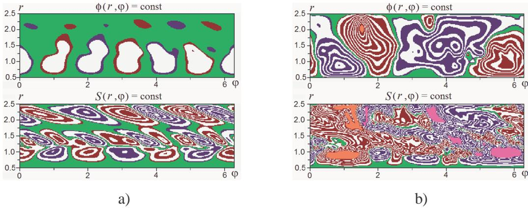
Fig. 1. 2D turbulent structures in levitated dipole system with external divertor separatrix in presence of sheared flows with uncontrolled vorticity: a) initial stage ( $t=8.5$ ) of partially suppressed turbulence; b) stage of well-developed turbulence ( $t=28.0$ ).
