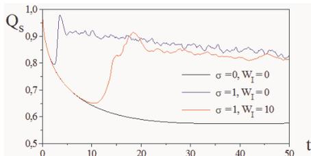
Fig. 2. Heat fluxes through the separatrix in regimes with low ( $W_I=0$ ) and high ( $W_I=10$ ) integral vorticities. Black curve presents regime without turbulence.
