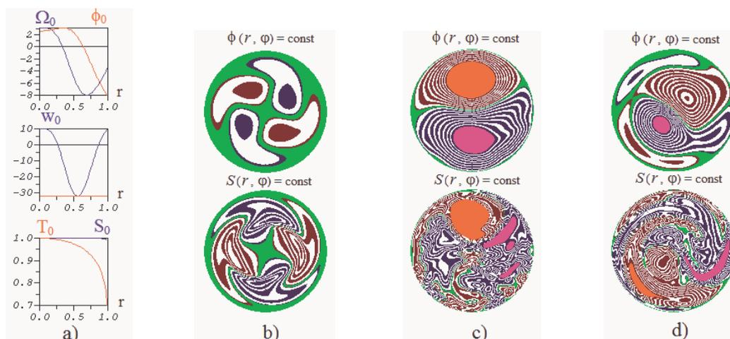
Fig. 4. 2D turbulent structures in tandem mirror central cell with divertor separatrix: a) initial radial profiles of plasma potential  $\phi_0$ , frequency of sheared rotation  $\Omega_0$ , dynamic vorticity of sheared rotation  $w_0$ , temperature  $T_0$ , and entropy function  $S_0$ ; b) initial stage ( $t=10.0$ ); c) well-developed turbulence with uncontrolled vorticity; d) well-developed turbulence with vorticity controlled by momentum source.
