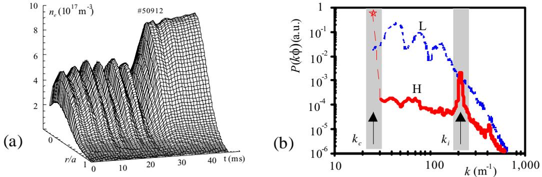
Figure 2. (a) Evolution of electron density during L-H transition in the H-1 heliac. (b) Modification to the spectrum of potential fluctuations from L to H mode.
