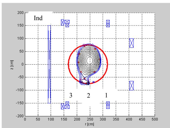
Fig.3 Poloidal field system of T15 with divertor
