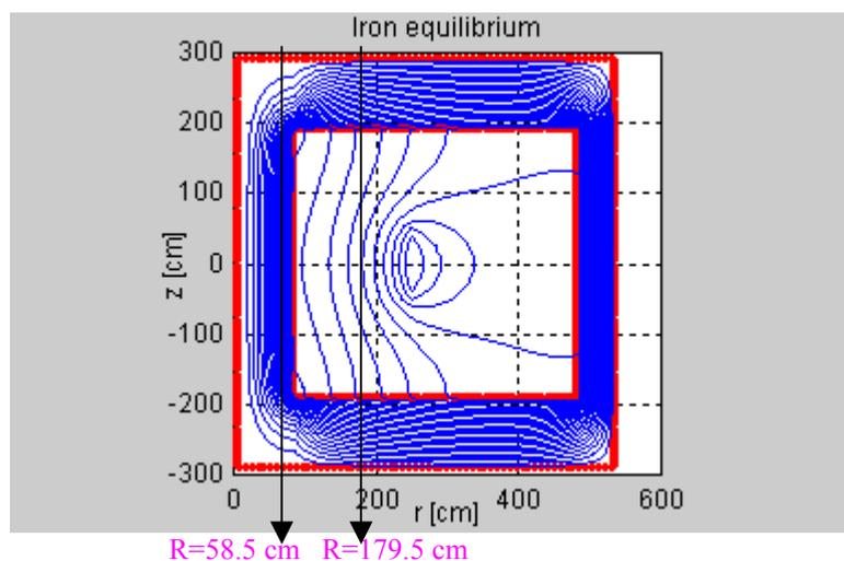
Fig. 1. 2D iron model approach in rectangular grid
