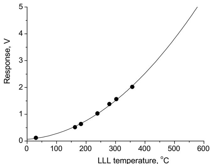
evaporation during the calibration procedure, which takes more than one hour per each channel. The calibration curve above this point is derived by extrapolation fitted to the blackbody response curve slope, assuming relatively small variation of Li surface emissivity in 350...600°C range.
