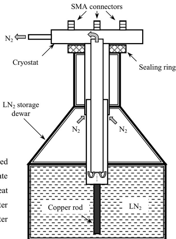
Fig.1. Schematic of immersion cryostat installed into LN<sub>2</sub> storage dewar. Arrows indicate evaporated N<sub>2</sub> flows for the proper heat recuperation and preventing air water condensation. Copper rod provides better cooling when LN<sub>2</sub> level is low.
