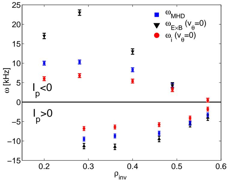
Figure 2: Comparison, in a safety factor scan, of the sawtooth precursors frequency  $\omega_{MHD}$  with the expected Doppler shift from the  $\mathbf{E} \times \mathbf{B}$  flow  $\omega_{E \times B}$  and the ion flow  $\omega_i$  (in case of pure toroidal rotation). Negative (positive) frequencies correspond to positive (negative) plasma current  $I_p$ .
