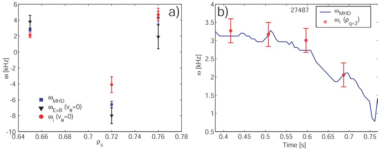
Figure 3: a) Comparison of TM and plasma flows rotation frequencies in case of isolated magnetic islands resonant with magnetic surfaces located at  $\rho_s$ . In details,  $m/n=2/1$  TM in L-mode with ohmic ( $\rho_s = 0.65$ ) and ECRH heating ( $\rho_s = 0.72$ ) and a  $m/n=4/3$  TM in H-mode with ECRH ( $\rho_s = 0.76$ ). b) a  $m/n=2/1$  TM in ohmic L-mode locking to the conducting wall.
