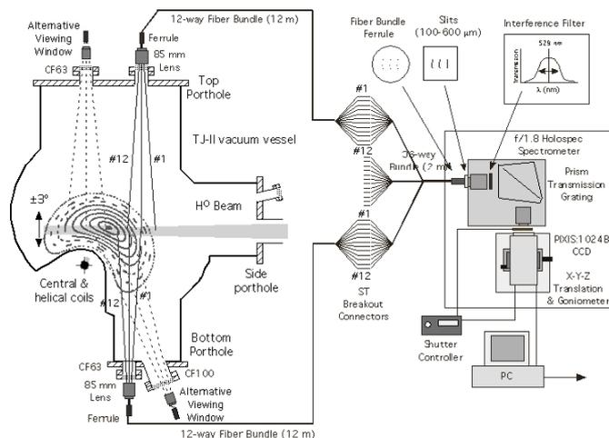
Fig. 1: Cross-sectional view of the TJ-II vacuum chamber and the DNBI.
