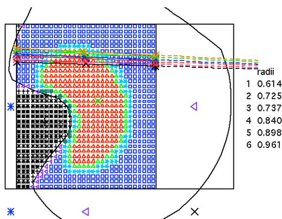
**Figure 1:** Poloidal section of the grid used for Eirene, with the 6 peripheral chords used in the Eirene simulation.
