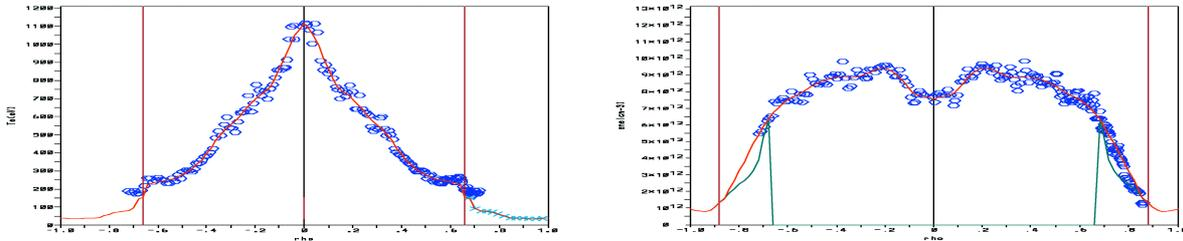
**Figure 2:**  $T_e$  (left, vertical scale from 0 to 1200 eV) and  $n_e$  (right, vertical scale from 0 to  $13 \times 10^{18} \text{ m}^{-3}$ ) radial profiles. Between the red vertical bars they are the symmetrised and smoothed Thomson scattering profiles. Beyond, the data are taken from a different, hydrogen discharge.
