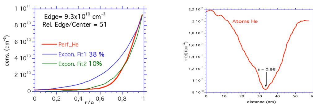
**Figure 4:** Neutral density profiles: radial profile inside the plasma, averaged over each magnetic surface (left); distribution along the 6<sup>th</sup> chord, the most external one (right).
