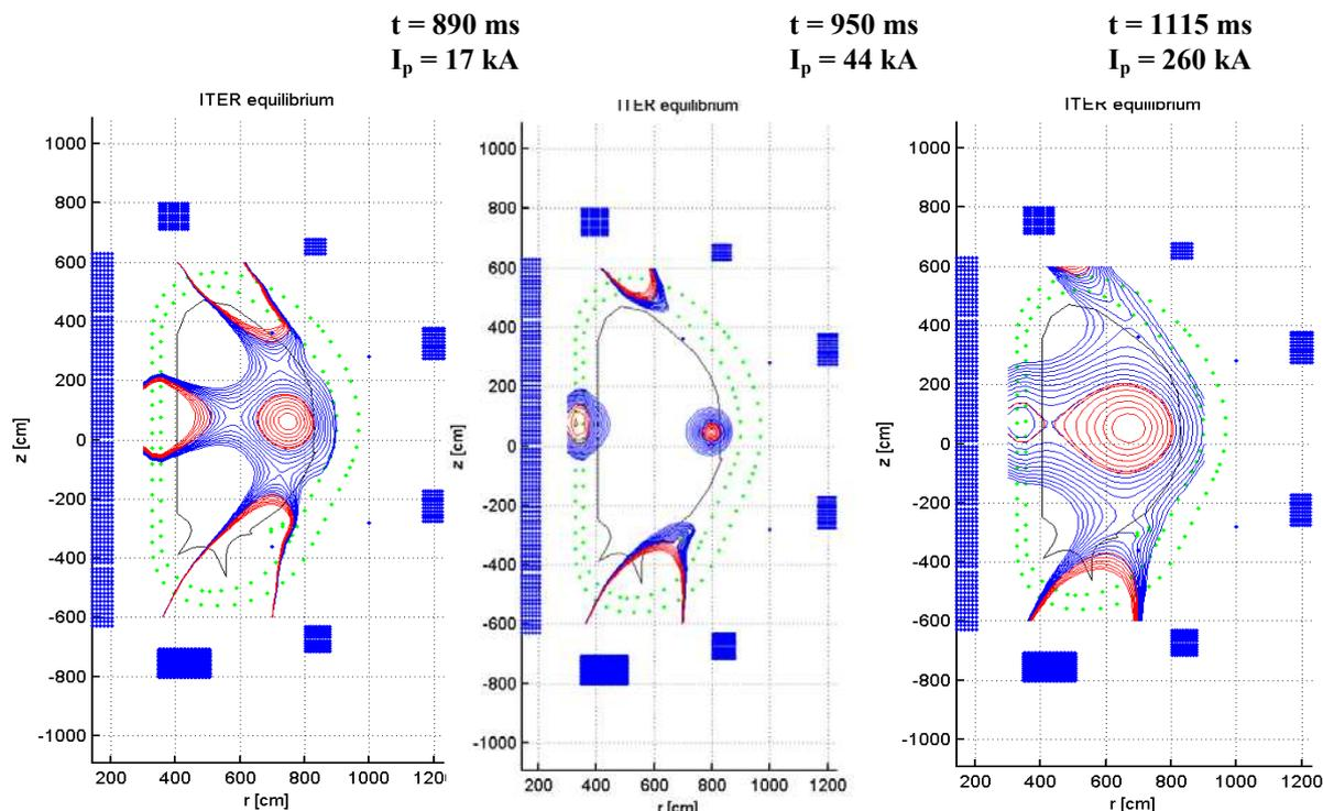
Fig.3 Plasma equilibrium in 890 ms time moment with prescribed PF coil currents from 0D modeling results (additional PF coil currents are not changed in time)
