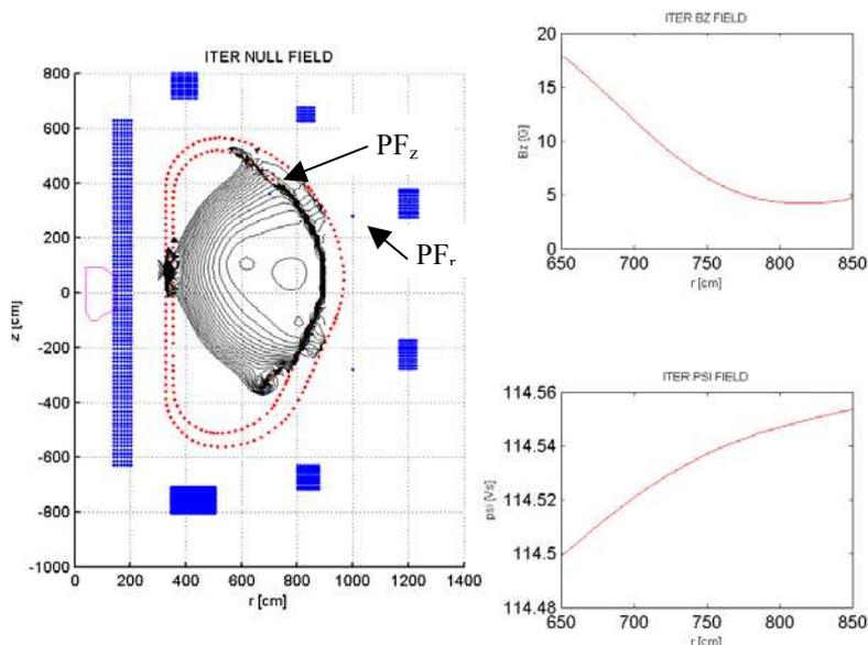
Fig.2 External magnetic field structure, radial dependence of  $B_z$  and  $\psi$  at time moment of plasma current formation ( $t = 850$  ms) without plasma with use of  $I_{PF}$  waveforms from 0D modeling.
