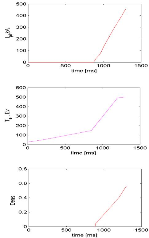
Fig.1 Time evolution of plasma current, electron temperature and plasma density during ITER plasma initiation
