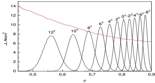
radial profile width, were deduced from the results of ECCD modeling and used for NTM modeling via modified Rutherford equation. The ECCD stabilization term  $\Delta'_{EC}$  in MRE is calculated according to Eq. (2) with substitution  $\tilde{j}_{bs} \rightarrow j_{ECCD}$ . With high accuracy, the driven current profile can be approximated by the Gaussian form
