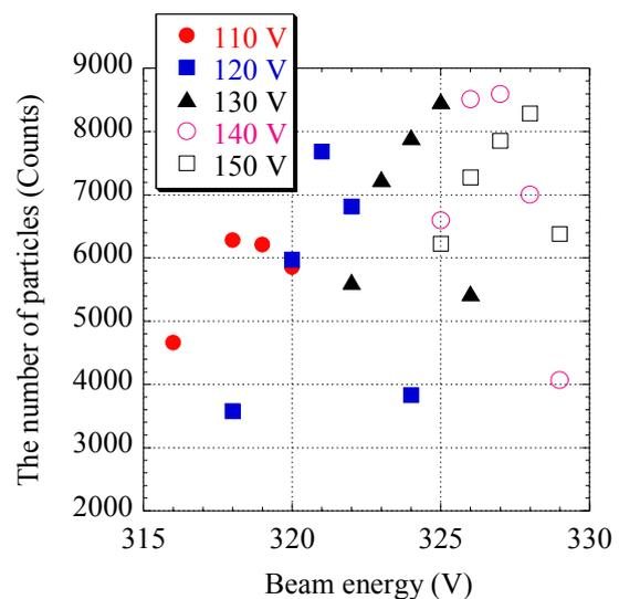
Fig. 2. The energy spectrum of HeH<sup>+</sup> particles measured by the mass spectrometer with energy analyzer for several arc voltages.
