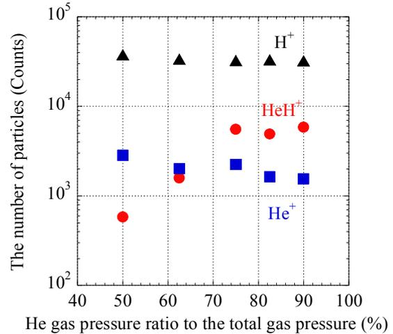
Fig. 3. The number of  $\text{HeH}^+$  (circle),  $\text{He}^+$  (square) and  $\text{H}^+$  (triangle) particles as a function of He gas pressure ratio to total gas pressure.
