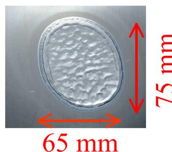
Fig. 5. The beam trace of the stainless steel target plate at  $X= 1530$  mm.
