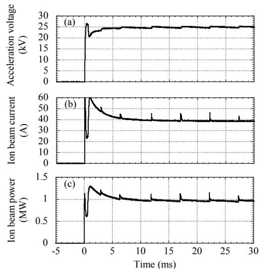
Fig. 4. Time evolutions of (a) acceleration voltage, (b) extracted ion beam current and (c) ion beam power.
