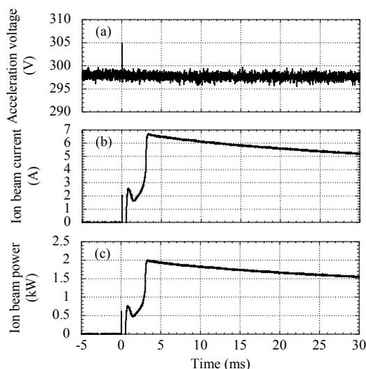
Fig. 1. Time evolutions of (a) acceleration voltage, (b) extracted ion beam current and (c) ion beam power.
