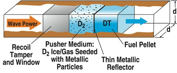
FIG. 1. The pellet-pusher module shown in a rectangular waveguide. Microwave power is transmitted through a transparent window, which also absorbs the pellet recoil momentum during acceleration.
