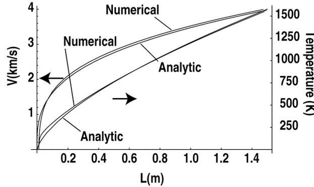
FIG. 2. Pellet velocity and pusher gas temperature as function of acceleration length obtained from numerical and analytic calculations
