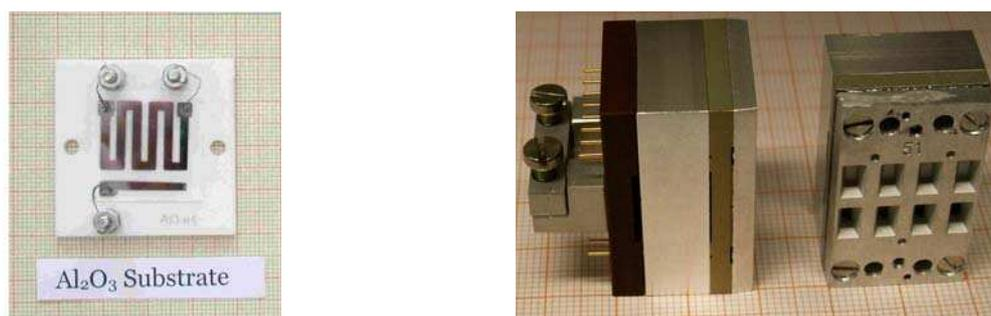
Figure 4. Left: sample of sputtered Pt deposited on alumina insulation successfully tested for  $\gamma$  and n irradiation. Right: a prototype bolometer with Pt - SiN meander-substrate to be irradiated in a neutron field.
