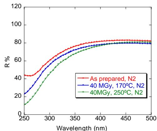
Figure 2. Degradation of reflectivity for  $\text{Al}_2\text{O}_3$  overcoated Al mirrors.
