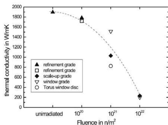
Figure 1. Degradation of thermal conductivity in high grade CVD diamond window due to n irradiation.
