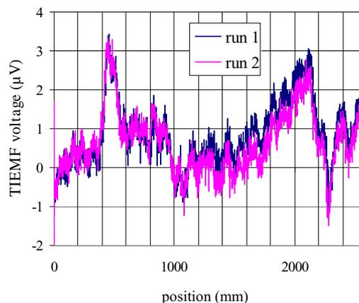
Figure 5. Dielectric constant of a PZ-type AFE thin film intended for a capacitive bolometer. Figure 6. TIEMF in MI cable heated to 300 °C.
