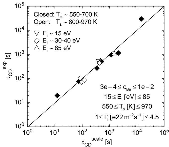
Fig. 1: Measured CD-emission decay time vs. empirical scaling given by eqn 1.
