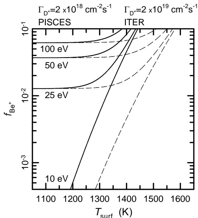
Fig. 2 – Conditions for tungsten beryllide formation in PISCES (solid lines) and predicted for ITER conditions (dashed lines). Beryllide formation occurs for conditions that lie above the ion energy curves.
