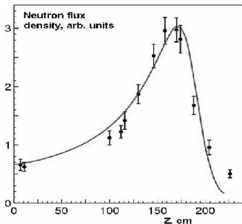
Fig.3 Axial profile of D-D neutron flux in GDT
