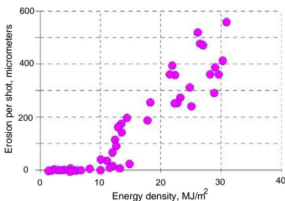
*Fig.1 The erosion depth of the graphite vs energy density*
