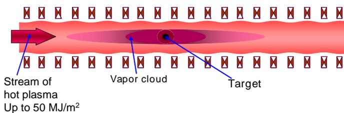
*Fig.2 Scheme of the experiment of carbon pellet injection into GOL-3 device*
