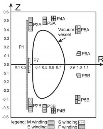
*Fig. 1 Poloidal coil system. The "M" windings provide the necessary plasma loop voltage control, the "E" windings adjust the plasma position and shape, the "S" windings provide the different plasma shapes, and the "F" windings provide feedback control of plasma position.*
