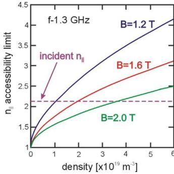
Fig. 5 LH slow wave accessibility (i.e. the condition for avoiding mode conversion from LH slow to fast wave) as a function of peak density and toroidal magnetic field.
