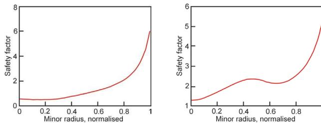
Fig. 4 Phase I, SNT, safety factor as function of radial position:
