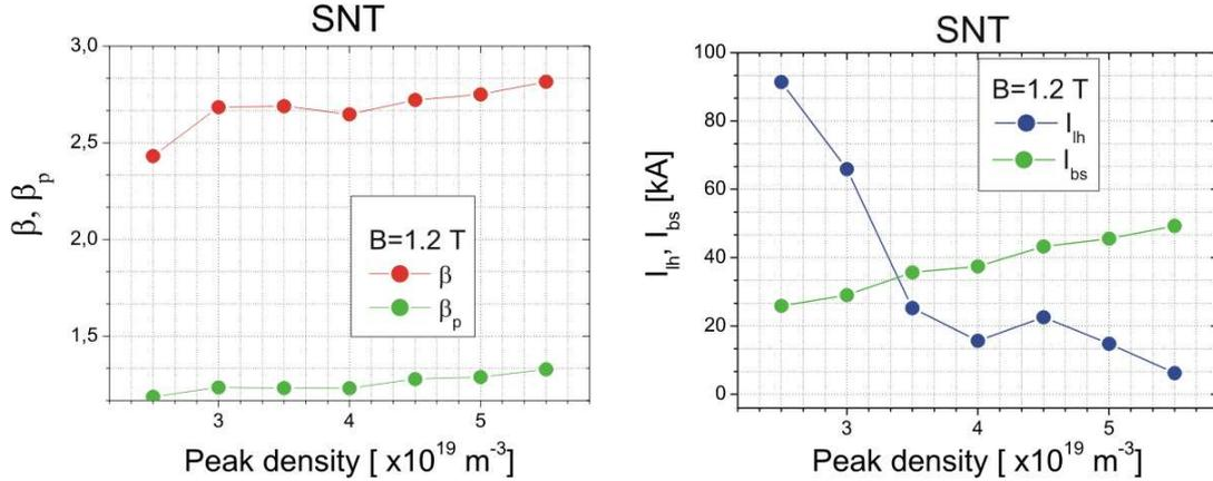
Fig. 3 SNT equilibrium,  $B_T = 1.2 \text{ T}$ ,  $I_p = 200 \text{ kA}$ , a)  $\beta$  [%] and  $\beta_{poloidal}$  versus peak density, b) LH current  $I_{LH}$  and bootstrap current  $I_{BS}$  versus peak density.
