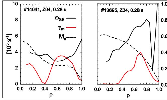
Fig. 3 Profiles of the ExB shearing rate  $\omega_{SE}$ , the growth rate of the most unstable ITG mode  $\gamma_m$  and the toroidal Mach number  $M_\phi$  for the two discharges shown in Fig. 1.
