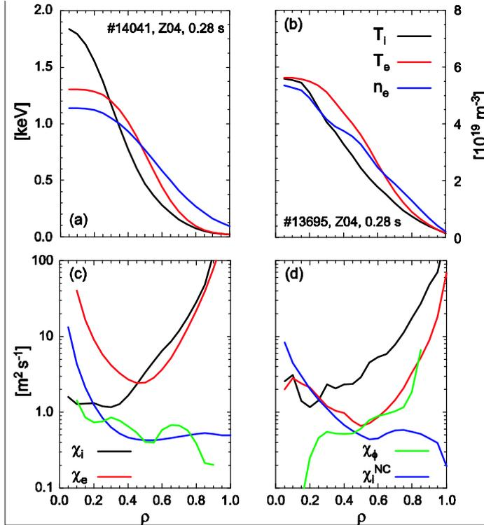
Fig. 1 (a) Profiles of  $T_e$ ,  $T_i$  and  $n_e$  vs normalised radius  $\rho$  during ITB discharges with co- (#14041) and counter- (#13695) NBI heating at 0.28 s and (b) the corresponding thermal,  $\chi_i$ ,  $\chi_e$ , and momentum,  $\chi_\phi$ , diffusivities from TRANSP analysis. The neo-classical ion thermal diffusivity  $\chi_i^{NC}$  from NCLASS is shown for comparison.
