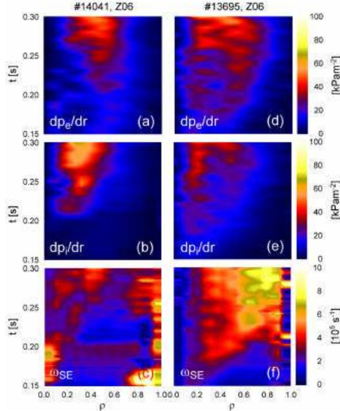
Fig. 2 Evolution of electron (a,d) and ion (b,e) pressure gradient and ExB shearing rate (c,f) profiles for the co- (a,b,c) and counter- (d,e,f) NBI heated discharges shown in Fig 1.
