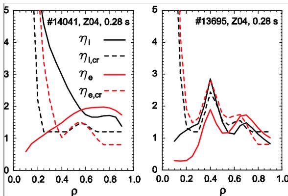
Fig. 4 Comparison of normalised ion and electron temperature gradients  $\eta_{i,e}$  with critical values for the de-stabilisation of ITG and ETG micro-instabilities for the discharges shown in Fig. 1.
