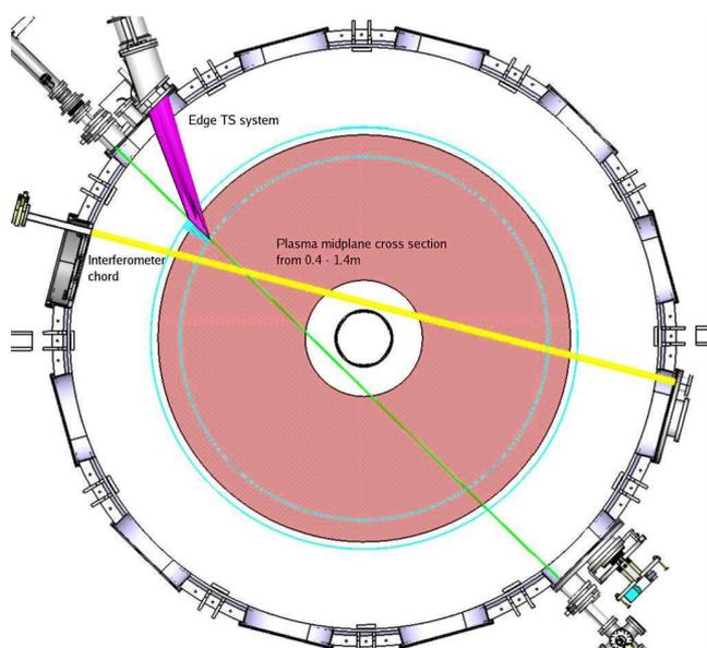
**Figure 1 - Plan view of edge Thomson scattering system optics and laser as well as interferometer chord. Plasma is shown with inner and outer radii of 0.4 and 1.4m and TS measuring between 1.29 and 1.45m.**
