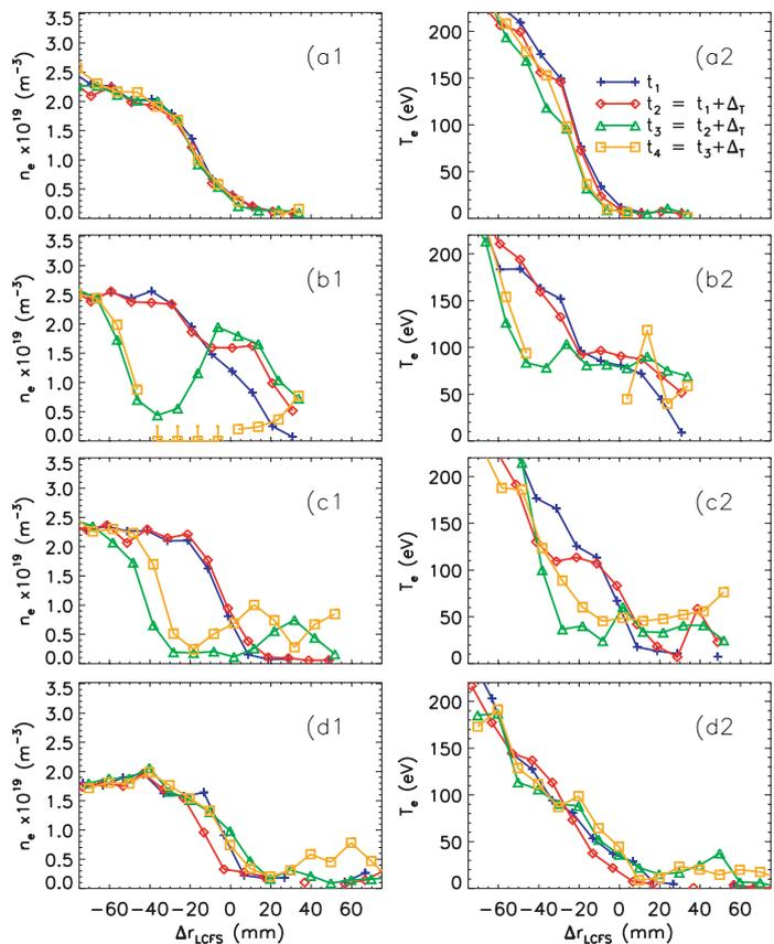
**Figure 2 - ELM filaments observed using lasers in burst mode 5μs apart. a) shows a profile obtained in an inter-ELM H-mode period, b-d) show filaments observed during ELMs classified according to distance of the filament from the pre-ELM last closed flux surface.**
