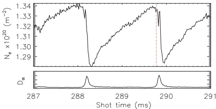
**Figure 4 –Single time point fluctuations seen during ELMs particle losses in interferometer data.**
