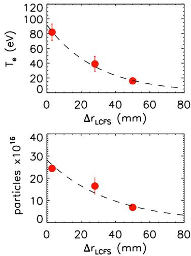
**Figure 3 – Filament temperature and number of particles plotted against filament center distance from the pre-ELM last closed flux surface.**
