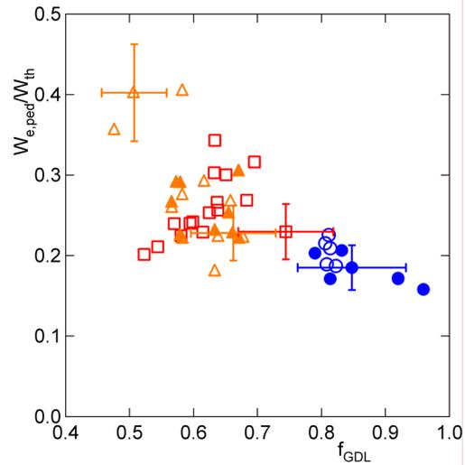
Fig. 3 : ratio of electron pedestal energy to thermal energy vs. density normalised to  $n_{GDL}$
