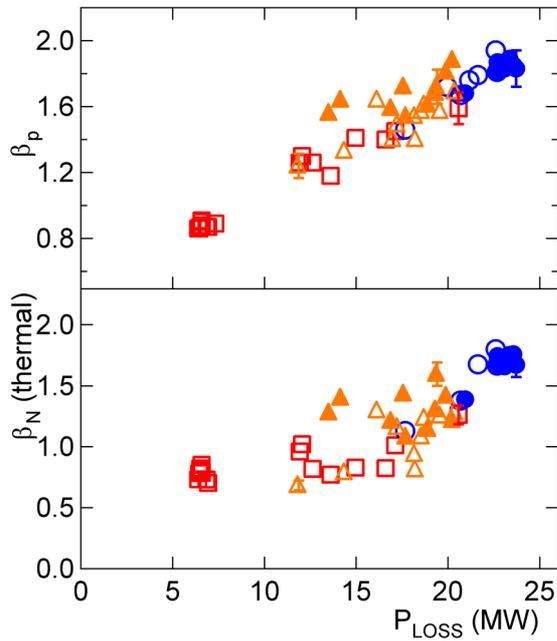
Fig. 1 : poloidal  $\beta$  and normalised  $\beta$  for the different scenarios in the dataset as function of loss power
