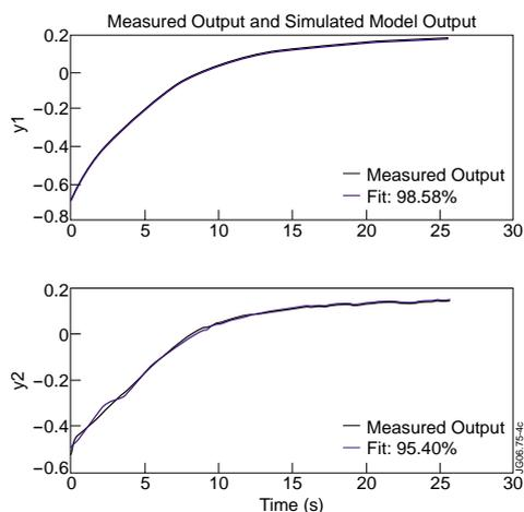
Fig. 3 Comparison between the free dynamics data from JETTO and from the identified state space (slow) model for two elements of the poloidal flux vector.
