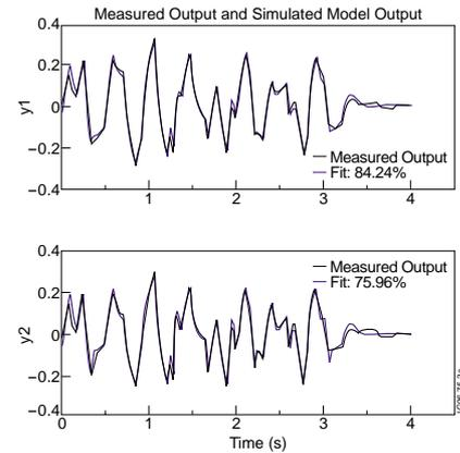
Fig. 2 Comparison between the data from JETTO and from the identified state space (fast) model for two elements of the electron temperature vector.
