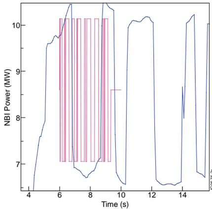
Fig. 1 Examples of a fast (red) and of a slow (blue) modulation of the NBI power used for the identification of a two-time-scale state space model.
