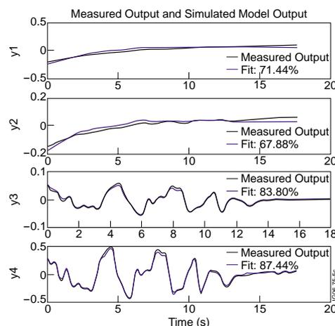
Fig. 4 Comparison between the data from JETTO and from the identified state space (slow) model for two elements of the poloidal flux vector and two elements of the electron temperature vector.
