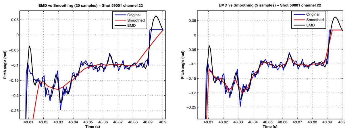
Figure 1 – Comparative performance between EMD and boxcar smoothing 20 ms (left) and 5 ms (right)
