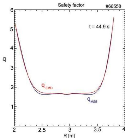
Figure 2 – Equilibrium reconstruction profiles with MSE data smoothed to 20 milliseconds (blue curve) and processed with the EMD technique (red curve) in 1 millisecond time scale.
