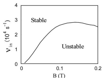
Fig. 1: Stability threshold of the  $(m, n) = (1, 1)$  mode on the  $B-v_{in}$  phase space.
