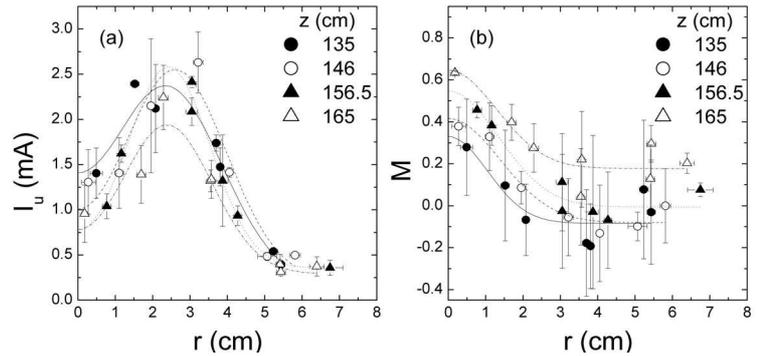
Fig. 3: Radial distributions of the ion saturation current detected by the upstream electrode of the Mach probe (a) and the Mach number (b) at several  $z$ 's.
