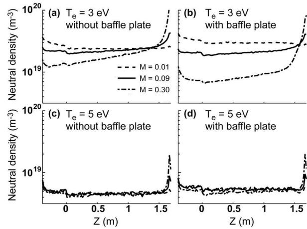
Fig. 2: Effect of Mach number,  $M$ , on the axial profile of neutral density at  $r = 2.5$  cm;  $T_e = 3$  eV (a, b) and 5 eV (c, d) without the baffle plate (a, c) and with the plate (b, d).
