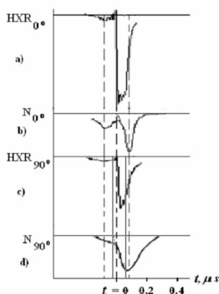
to it (*c*,  $90^\circ$ ) they are moved forward by their time-of-flight (TOF) of the 7-m distance (23.3 ns). Neutron pulses seen in the picture provide data on powerful streams of fast (also  $\sim 100$  keV) ions.
