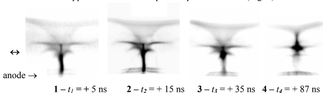
Fig. 3 Experimental images of the current cutoff phenomenon (marked by a sign ↔) taken by the optical image camera with 1-ns time resolution
