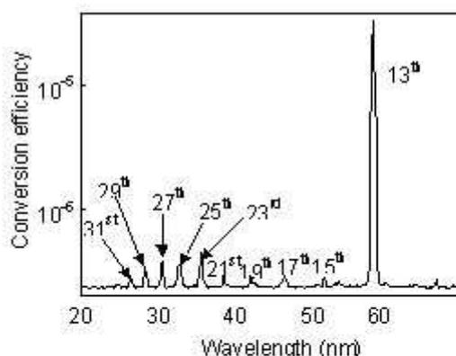
**Figure 4** Spectrum of the high order harmonic generation was obtained using the indium plasma. The conversion efficiency of 13<sup>th</sup> harmonic is  $8 \times 10^{-5}$ .
