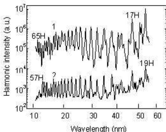
**Figure 1.** Harmonic output as a function of the wavelength of generated XUV radiation in the cases of (1) boron and (2) silver.
