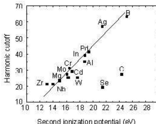
**Figure 2.** Dependence between the cutoff harmonic and ionization potential of ions (second ionization potential) for different targets.
