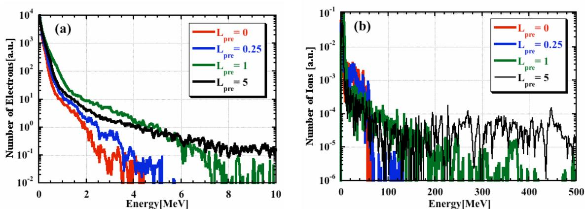
Fig. 3 (a) Time averaged electron energy spectra at Obs1, and (b) time averaged ion energy spectra at Obs2 for  $L_{pre}=0, 0.25, 1$  and  $5$  [ $\mu\text{m}$ ].
