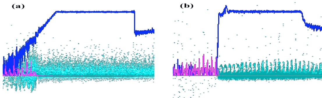
Fig.2 Electron phase space (light blue), electron density (blue) and laser field (purple) at  $t=1000$  [fs] for (a) immobile ions and (b) mobile ions.
