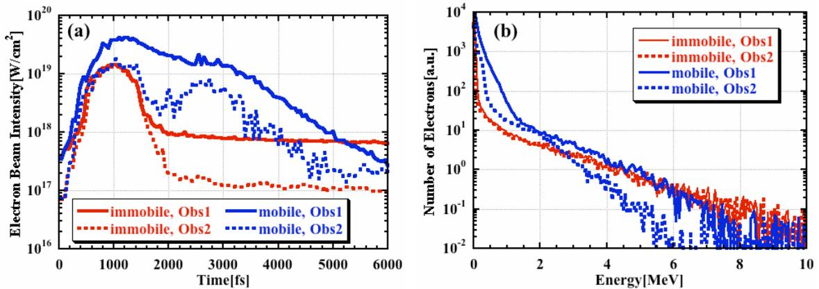
Fig.1 (a) Time evolution of electron beam intensity and (b) time averaged electron energy spectrum for immobile (red) and mobile (blue) ions. Solid lines are corresponding to Obs1, and dash lines to Obs2.
