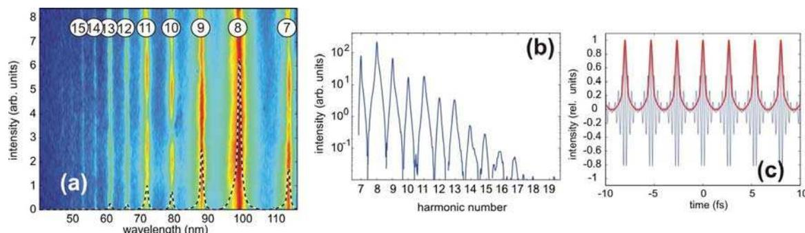
Fig. 3: (a) experimentally produced harmonic spectrum using Quartz targets. (b) the harmonic comb in frequency domain. (c) the train of attosecond pulses ( $\sim 400$  as) assuming that the frequency comb in (b) is coherent.
