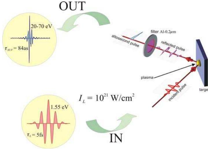
Fig. 1: Schematic showing the technique of attosecond pulse generation from the interaction of high-intensity laser pulse with solid targets.
