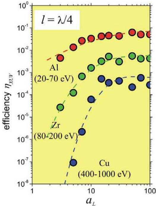
Fig. 2: The efficiency of the laser to attosecond XUV pulse conversion as a function of the normalized field amplitude for three different filter materials (1D-PIC simulations).
