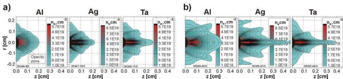
Fig. 2. Electron isodensitograms at  $\Delta t=17 \text{ ns}$  for different target materials correspond to: a) the first and b) third harmonic of the laser radiation.
