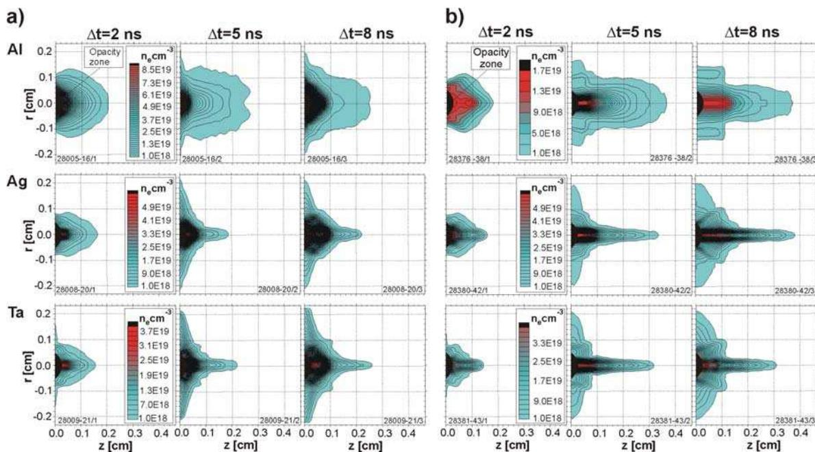
Fig.1. Sequences of electron isodensitograms for different target materials correspond to: a) the first and b) third harmonic of laser radiation.
