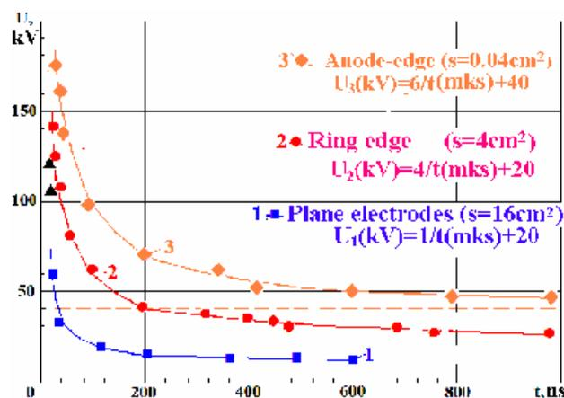
Fig.7. Pulse duration as a function of the hold-off voltage for various types of electrodes
