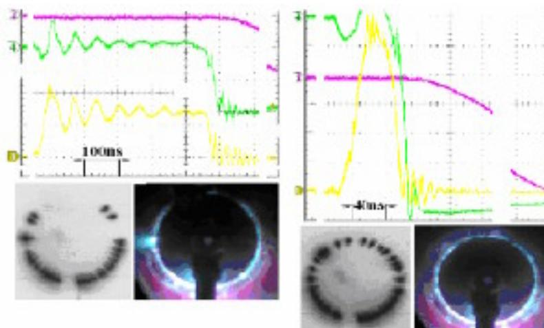
Fig. 6 Top: 1 – voltage (25 kV/div), 3 –  $dI/dt$  signal ( $8 \times 10^9$  A/div), 4 – current (12.5 kA/div). Bottom: electron image frame 100 ns after current beginning and integral photo.
