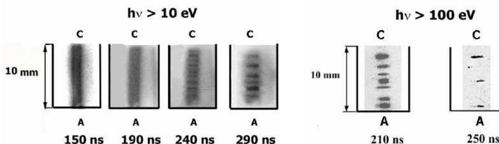
Fig. 4. ICT photographs of the plasma surrounding the central electrode in the SXR range.
