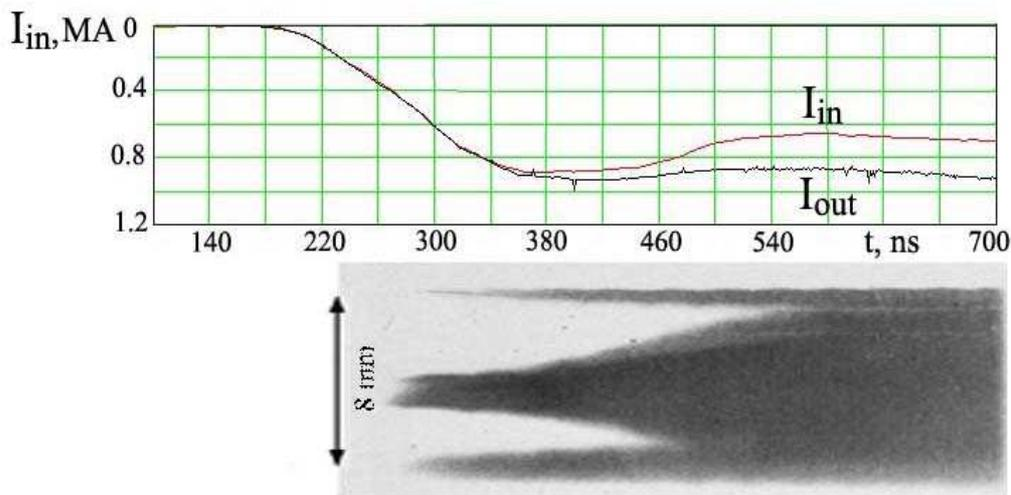
Fig. 3. Top: oscillograms of the input ( $I_{in}$ ) and output ( $I_{out}$ ). Bottom: chronogram of the plasma expansion in the MITL model (the negative).
