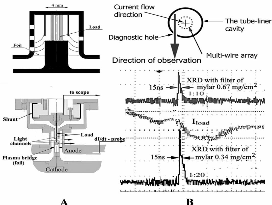
Fig. 1. A – Principal and experimental schemes of the plasma flow switch output device; B – wall temperature measurements on the base of SXR signals
