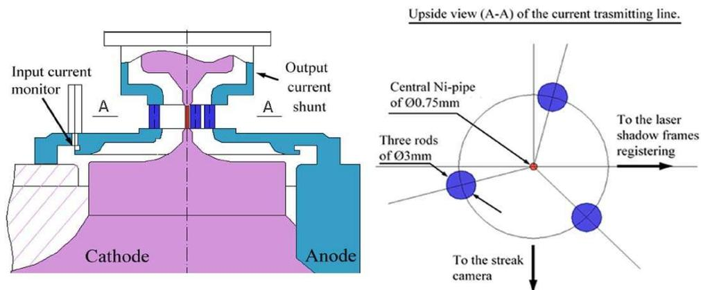
Fig. 2. Scheme of the MITL experiment with a shunt.
