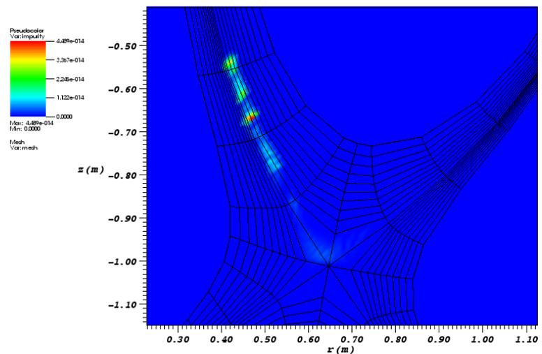
Figure 2: Impurity deposition for micron radius graphite grains in MAST.
