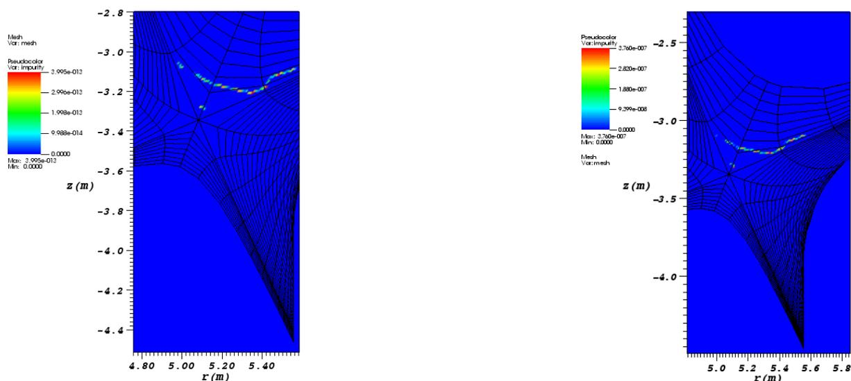
Figure 3: Impurity deposition for 1 micron (left) and 100 micron (right) radius tungsten grains in ITER.
