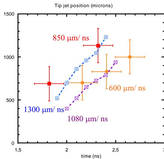
Figure 3 : Tip jet position in experiment and 2 simulations with different heat transport model
