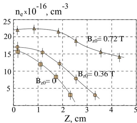
Fig. 1. Plasma shield density vs. the distance from the target surface (25 MJ/m<sup>2</sup>,  $\Delta\tau = 20$   $\mu\text{s}$  from the beginning of plasma interaction with the surface).
