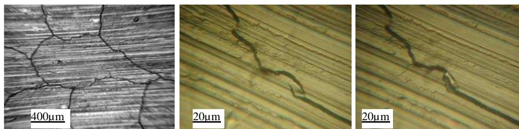
Fig.5. Mesh of cracks at the tungsten surface, crack bifurcation, and melting of the separated piece.
