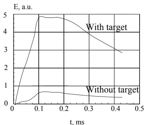
Fig. 3. Intensity of the shielding layer radiation measured with  $\text{LiNbO}_3$  detector.
