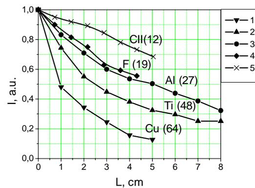
Fig.2. Spatial distributions of evaporated materials in front of the surface for different exposed targets evaluated from spectral lines: CuII (2590Å), TiII (4534Å), AlIII (5593Å), FII (4109Å) and CII (4267Å).
