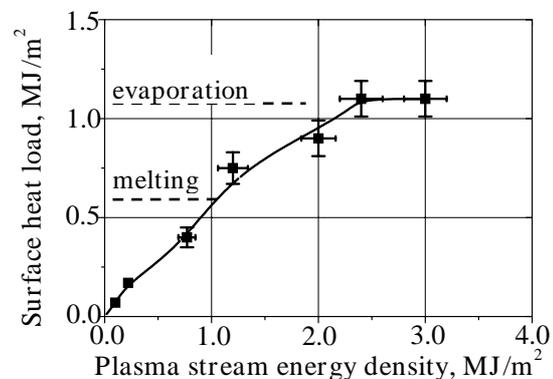
Fig. 4. Heat load to the tungsten surface vs. energy density of impacting plasma stream.
