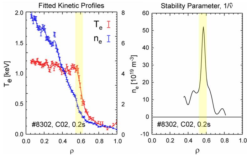
Fig 5: Experimental values of  $1/\hat{v}$  in a MAST ITB
