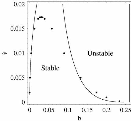
Fig 1: Critical  $\hat{v}(b)$ ; numerical (dots), asymptotic limits (lines); vertical line is eqn.(4)
