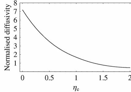
Fig 4: Variation of  $\hat{D}$  with increasing  $\eta_e$  implying inward thermo-diffusion ( $\hat{v} = 10^{-3}$ )
