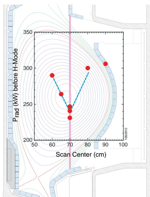
*Fig. 3 Radiated power just before the H-mode transition as a function of boronization deposition location prior to each discharge. Superimposed is a typical equilibrium reconstruction for the tokamak plasma. The vertical line shows the EC resonance for the cases at  $R=70$  cm.*
