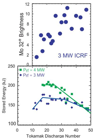
Fig. 2 a) Increase in Mo radiation from the core plasma for a sequence of tokamak discharges following an overnight boronization; b) Corresponding trends in stored energy for 2 levels of ICRF auxiliary power
