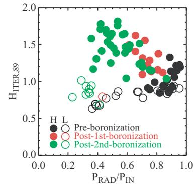
Fig. 1 Energy confinement enhancement vs. radiated power fraction for L- and H-Mode discharges, pre-and post boronization
