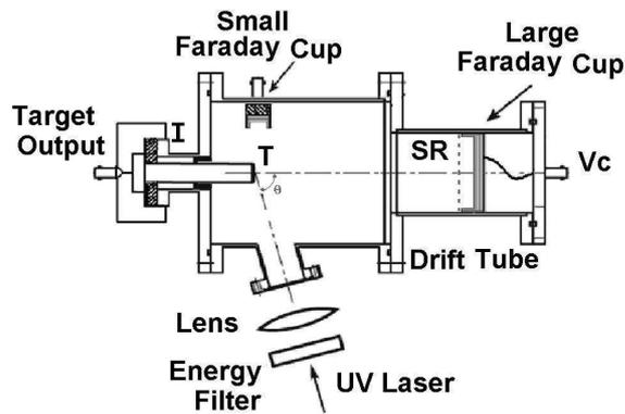
**Fig. 1.** Experimental apparatus. The laser beam axis was tilted of  $70^\circ$  with respect to the chamber axis.
