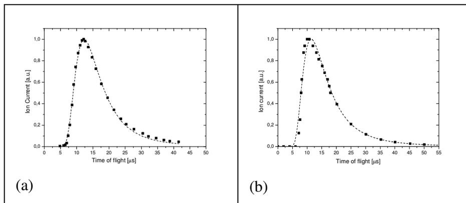
**Fig. 2.** a): Ion current waveform recorded by the axial FC. The dash line represents the best fit curve by Eq. (1.5). b): Ion current waveform recorded by the radial FC. The dash line represents the best fit curve by Eq. (1.6).
