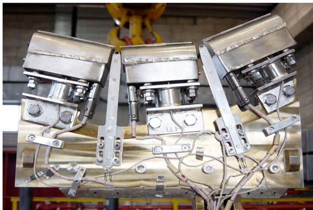
**Fig. 1.** Photograph of the three units of Liquid Lithium Limiter installed on the support used for the LLL introduction inside FTU.
