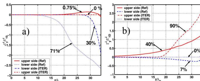
Figure 3: Vertical ion flux falling on the sides of the gap for poloidal (a) and toroidal (b) cases normalized to the non-perturbed influx flowing onto tile surface for the case ( $20^\circ$ ,  $1 \text{ mm}$ ) and ( $5^\circ$ ,  $0.5 \text{ mm}$ ). The percentages correspond to the total incident current normalized by the sheath edge current density integrated across the gap entrance.
