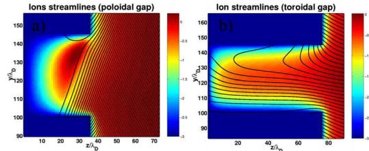
Figure 2: Ion streamlines in the case of poloidal (a) and toroidal (b) gaps plotted over the electric potential normalized to  $kT_e/e$  for the reference case, i.e., an angle of  $20^\circ$  and a gap width of  $1 \text{ mm}$ .
