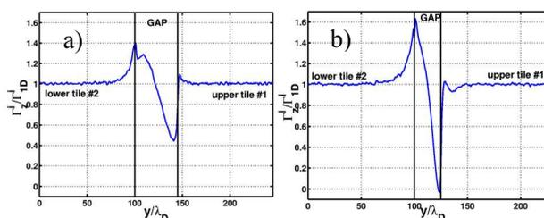
Figure 5: Horizontal ion flux normalized to the non-perturbed influx flowing onto tile surface along the vertical coordinate at the gap entrance for a toroidal gap for a) reference case ( $20^\circ$ ,  $1mm$ ) and b) ITER ( $5^\circ$ ,  $0.5mm$ ).
