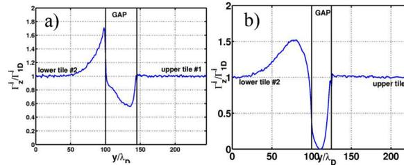
Figure 4: Horizontal ion flux normalized to the non-perturbed influx flowing onto tile surface along the vertical coordinate at gap entrance for a poloidal gap for a) reference case (20°, 1mm) and b) ITER (5°, 0.5mm).
