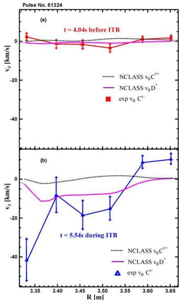
Figure 2: Comparison between measured  $v_\theta$  and neoclassical predictions both for impurities and main ions, (a) before and (b) during the ITB phase.
