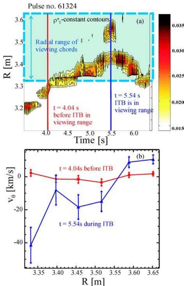
Figure 1: (a) Dynamics of the ITB and region covered by the  $v_\theta$  diagnostic. (b)  $v_\theta$  profiles before and during the ITB.
